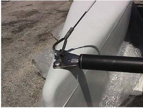
**1** Before installing the jib on the Hobie Wave, you must first install the parallel bow spreader (provided with the turbo kit). Install bow spreader tangs on each bow under existing bridle wire tang as shown. Pin faces towards center. With trampoline loosened, place bow spreader in position on pins installed on bows.
