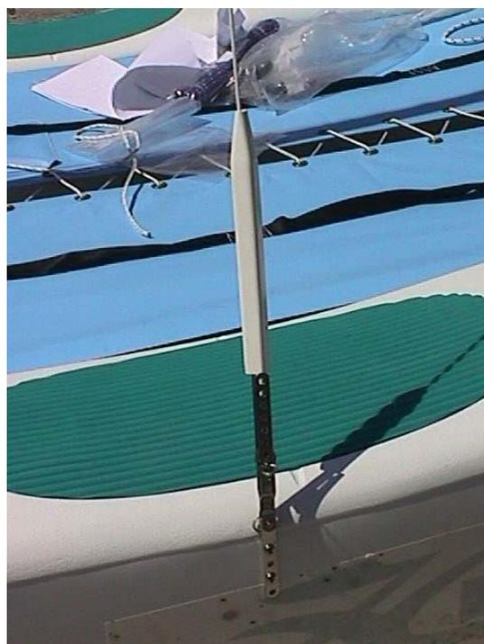
Next, fasten the shrouds into the stay adjusters. To begin with, fasten the shroud about half way up the adjuster. This position can be adjusted later. The position influences mast rake. Now fasten the twist toggles to the anchor bar pins on each side of the boat. You can pull the cover partially over the stay adjusters at this time. The assembly of the trapeze wires can wait until after you have raised the mast.
