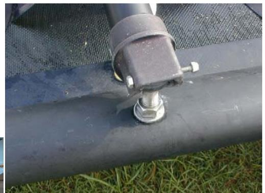
Once the mast is standing and the wires all attached remove the nut and bolt from the mast base. This is only necessary for raising and lowering the mast.
