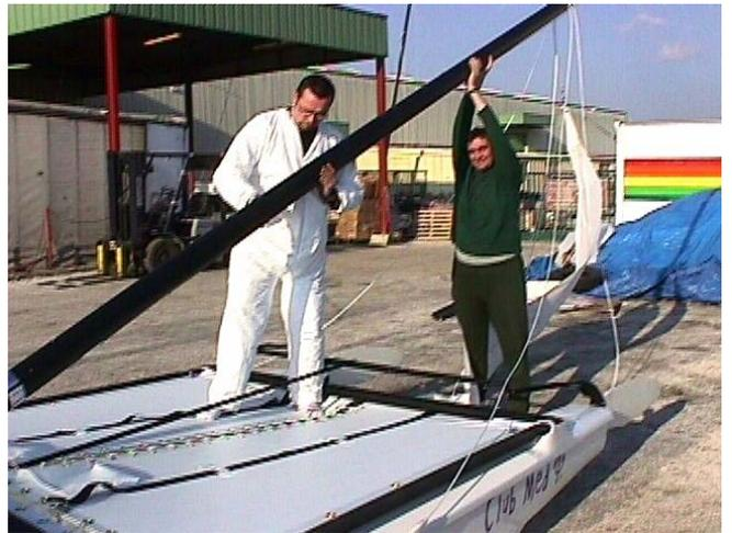
The second person moves to the front of the boat and attaches the forestay to the top hole in the furler chainplate. Now the jib tack is attached to the chainplate using the shackle provided.
