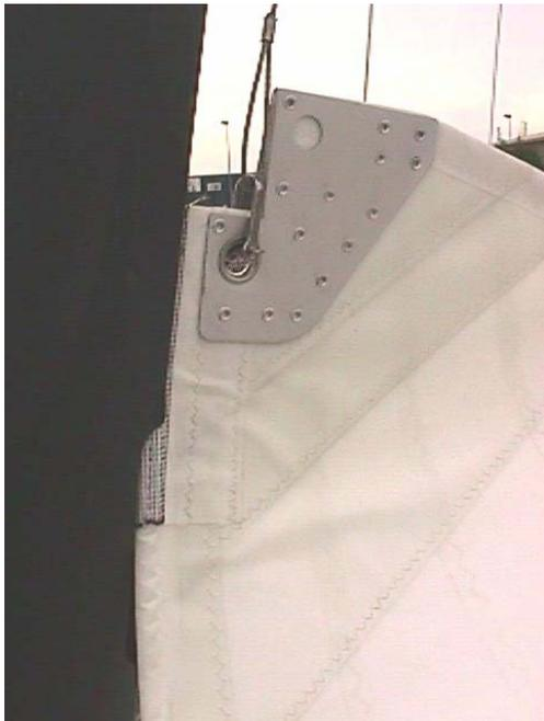
**2** Position the boat so that it is facing into the wind. Attach the main halyard shackle to the headboard of the mainsail. Feed the bolt rope into the mast cut out.
