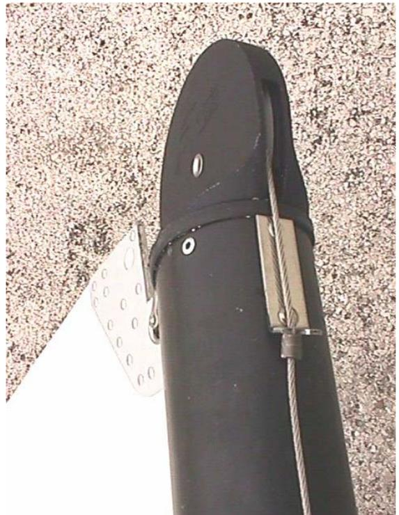
**4** When the sail is all the way to the top of the mast, engage the slug on the halyard wire into the halyard lock. Secure the halyard line to the cleat on the side of the mast. Stow the excess line in one of the trampoline pockets.
