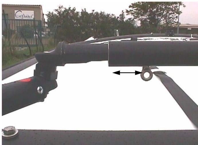
**1** Assemble the stay adjusters with twist toggles, clevis pins and split rings. Attach them to the anchor bar pins. Ensure that the stay adjuster points fore and aft - as per photograph.
