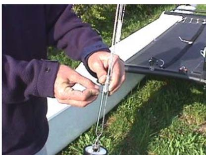
**10** With the person on the trampoline supporting the mast, the other person takes the forestay and connects it to the stay adjuster fixed to the jib furler. Pin the forestay towards the top of the adjuster. Now, provided all the clevis pins have the split rings fitted, the mast is supported by the shrouds and forestay.
