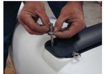
**4** Pass your hand through the inspection port to position the nuts and washers onto the long bolt and the headless bolt.
