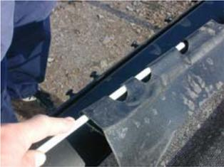
**2** trampoline in the centre. Pull the trampoline to the back of the boat and insert the fibreglass rod into the rear flap of the trampoline. Leave an equal amount protruding from
