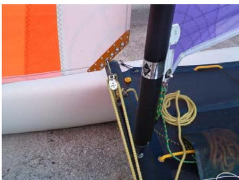
**3** Attach the jib clew blocks to the clew of the jib using the snap hook provided.
