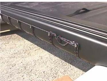
**7** edge of the trampoline and tie off securely. Repeat procedure for port side. Retighten rear lacing from left to right. Tie the rear lacing off securely at the eyelet posts on the right hand end of the rear beam. **NB :** It is important that the trampoline lacing is kept very
