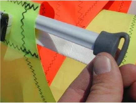
**1** Unfold the mainsail and lay on a flat clean surface. Undo the set of battens and identify which batten goes in which batten pocket. Insert the battens into the pockets.
