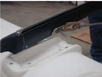
**3** Taking the front crossbar, position it on the crossbar moulding in the deck making sure that the eye strap on the bar is facing to the rear of the boat and the remaining headless bolt on the cross bar fits in the hole on the deck. Insert the long external screw.
