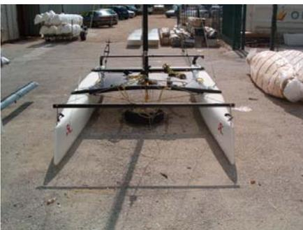
**4** Locate the Jib furler and shackle it to the bridles using the 6 mm shackle provided. Ensure that the exit hole in the furler is pointing at the furler cleat on the front crossbar. Check that the screw on the underside of the furler is tight. This prevents the outer cover from rotating.
