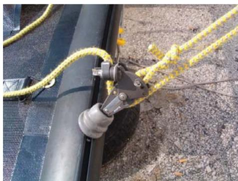
**4** Thread the jib sheet line through the jib sheet blocks. Fasten the sheet to the top of the blocks using a bowline knot. Ensure that there are no twists in the sheet and that the sheet is led behind the mast.
