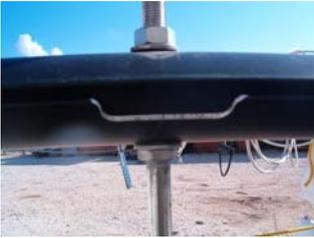
**1** Unfold the trampoline. Note that the side tension lines are prethreaded. Insert the front sealed bolt rope edge into the trampoline track of the front crossbar. Continue feeding the trampoline into the trampoline track and position it in the centre. Line up the grommet in the centre of the front edge of the trampoline with the dolphin striker post. This will position the
