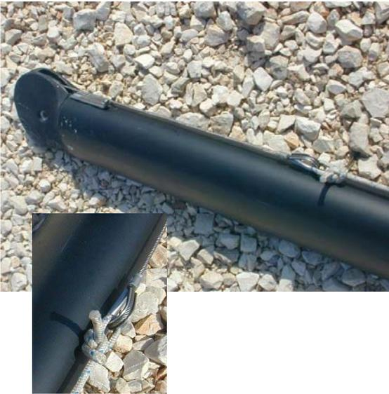
**1** Remove the main and jib halyard lines from the ropes bags. Unroll the main halyard wire that is secured at the head of the mast. Using a bowline knot, secure the main halyard line to the thimble at the end of the halyard wire. Now, secure both ends at the base of the mast.
