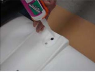
**2** Lift the right hull into an upright position. One person straddles the hull to hold in position. The other one applies the silicone sealant (for waterproofing) around the bolt holes and on rivets.
