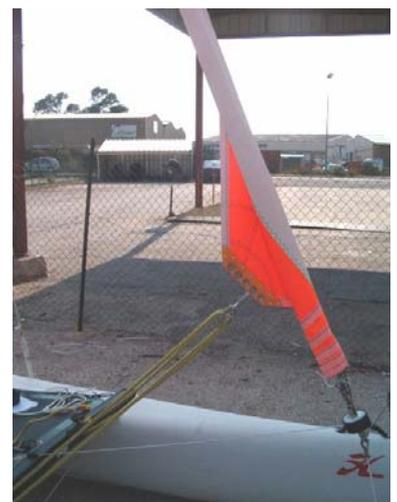
**5** The jib can now be furled by pulling on the furler line and cleating it off in the jam cleat. The jib will not furl fully if the jib sheet is cleated on.
