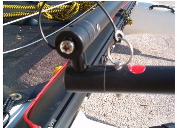
**4** Locate the tiller crossbar and identify the left and right hand ends. NB: the tiller crossbar (1) locates on top of the tiller/rudder arms (2).
