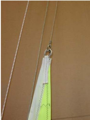
**1** Unfold the jib and shackle the head onto the jib halyard with the shackle provided. Fasten the clip at the top of the jib to the forestay wire. Pull on the halyard and raise the sail, fastening each clip to the forestay in the process. When the sail is raised, shackle the tack of the jib to the adjuster on top of the furler. Fasten as low as possible.
