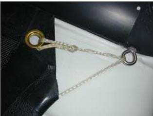
**4** Tensioning the sides : starting at the right rear corner, take the line that emerges from the trampoline. Lead it through the eye strap on the rear beam and then through the grommet/eyelet. Tie it off with a bowline knot or similar.
