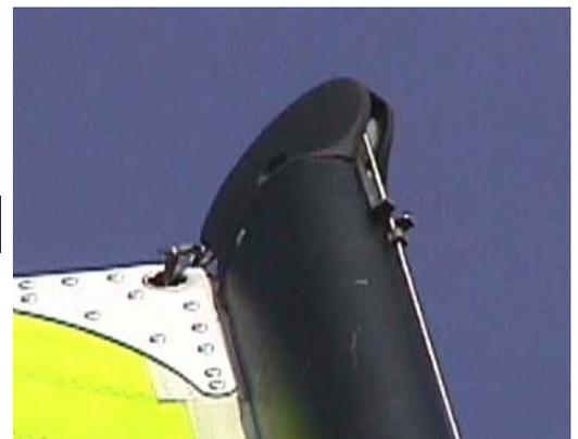
**6** position the stopper on the wire halyard so that it engages in the halyard lock.
