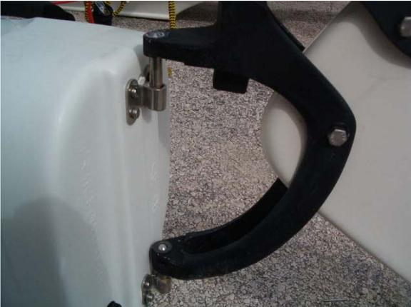
**1** Identify the right rudder from the left rudder (look for the stickers on the rudder arms). As shown, line up the rudder pintles (metal pegs on the hulls) with the rudder castings. Push the rudder castings down onto the pintles.
