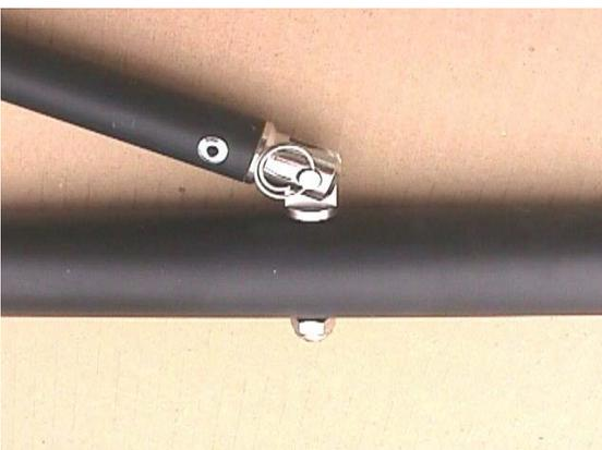
**5** Locate the tiller extension and secure it to the tiller crossbar using the clevis pin and ring clip provided.
