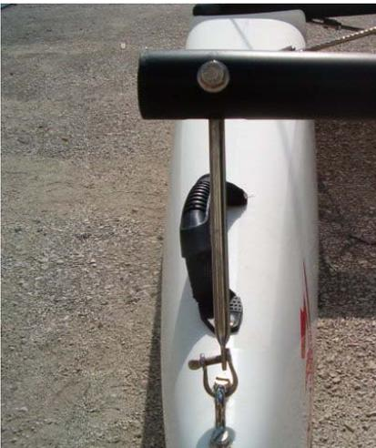
Identify the right side from the left side of the bar (look for the stickers) and position it the right way between the two hulls and attach the bar with the supplied shackles as shown on the photo.
